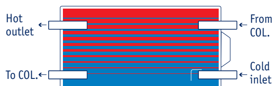
Solar (Open-Loop system)
