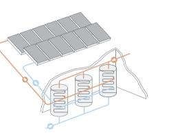
Hospitals require high water temperature for various needs such as Operating rooms, laundry, dining rooms, kitchen and showers. The hot water generated by the collectors is stored in storage tanks, and distributed within the building. The older conventional heating system may work as a back-up system. The system is designed to prevent legionella in hospitals projects.
